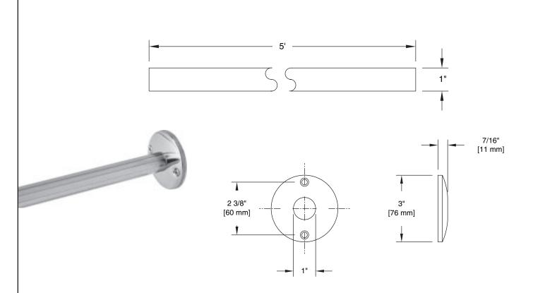
MATERIALS: 161 tubing is of 1" O.D. x .035 (20 gauge) seamless type 304 polished stainless steel. 162 tubing is of
